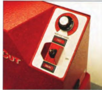
2. CONTROL PANEL is positioned to provide easy access and view of disc / drum selector switch and feed speed control knob.
