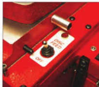
8. INDICATOR LIGHTS on disc and drum feed and selector switches help ensure simple safe operation for technician.
